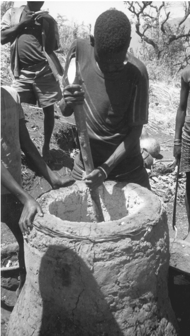
Figure 5. The bloom is recovered from the furnace with an iron pick (photo. Randi Haaland).
