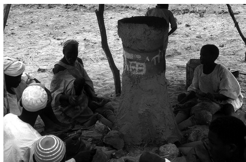
Fig. 4. Fur blacksmiths are starting to blow the bellows during the early part of the smelting operation. Note the figures drawn on the shaft furnace. Photo G. Haaland.
