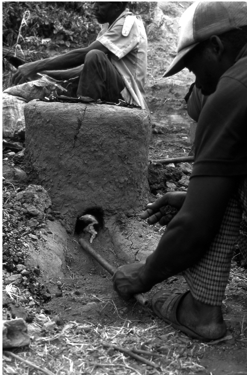
Fig. 6. Slag is starting to flow from the small blast furnace. Photo R Haaland.
