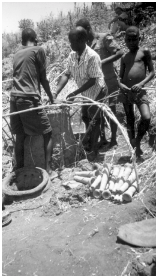
Fig. 4 Chilaco inspecting the furnace made ready for smelting; note the pot-bellows and tuyeres in front of the furnace. (photo Gunnar Haaland)
