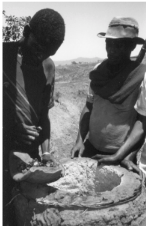
Fig. 6. Chilacho inspecting the bloom taken out of the furnace (photo Randi Haaland)
